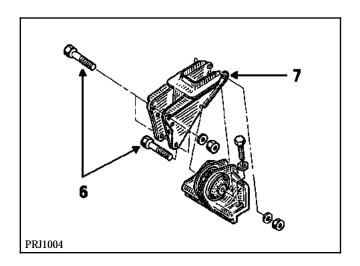
Remove the two mounting bolts from the power assisted steering pipe on the sub-frame.
