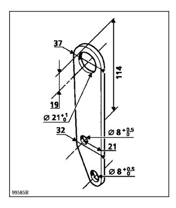
There are two ways of making this lifting bracket.
