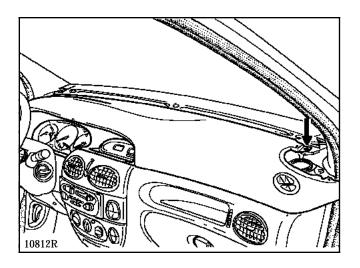
Unclip it, lift it up and remove towards the front of the vehicle.
