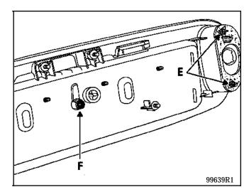
Remove the fog light(s) by slackening the two nuts (E).
