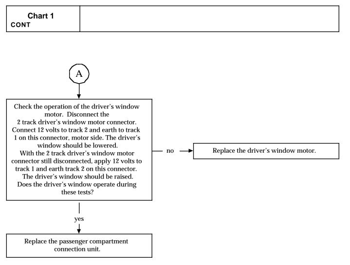
Check the driver's window operates correctly.
