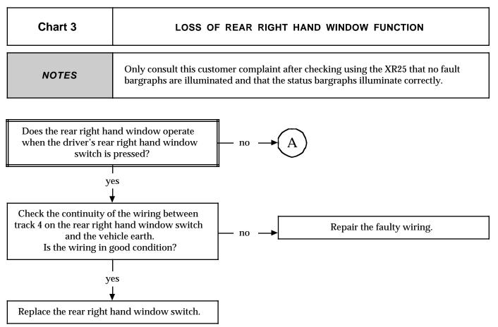
Check the rear right hand window operates correctly.
