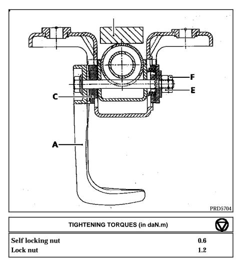
Fit a 15 mm thick shim between the body and its mounting, so that it is set vertically and the adjustment system may then be tightened later on.
