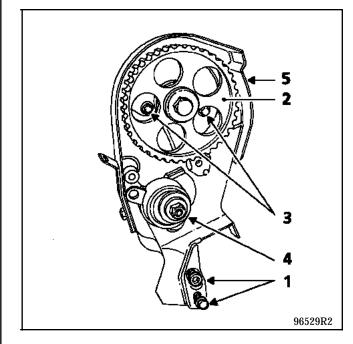
Remove the inner timing cover (5).
