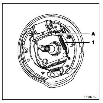
Fit a clamp on the wheel cylinder pistons.
