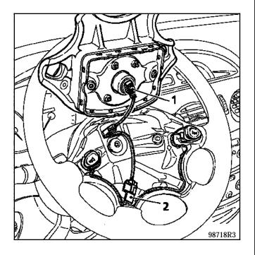
Immobilise the rotor of the rotary switch under the steering wheel using adhesive tape.
