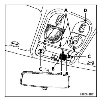
Remove the two mounting bolts (C) and release the roof console towards the front of the vehicle.
