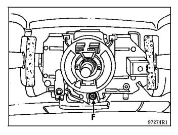
Slacken bolt (F) so that the control stalk assembly may be removed.
