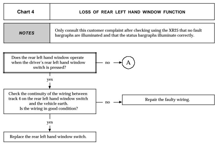
Check the rear left hand window operates correctly.
