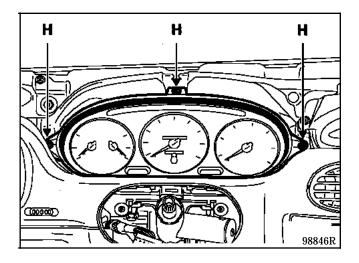
Remove the instrument panel, three bolts (H).
