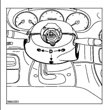
Remove the half cowling under the steering wheel by the three bolts (D).
