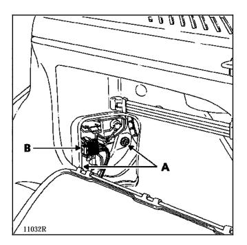
Slacken the two mounting nuts (A) on the rear lights unit and release the unit to the outside after disconnecting the connector (B).
