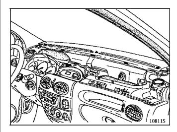
Release the instrument panel and disconnect the connectors.
