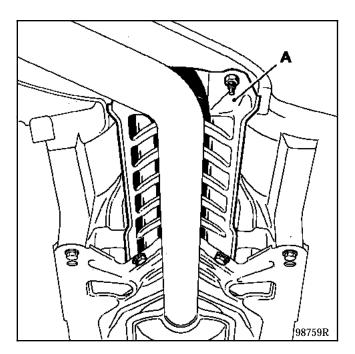
the rubber mountings for the exhaust pipe,
