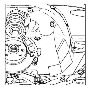
Remove the screen wash bottle from its mounting (F) after having disconnected its wiring.
