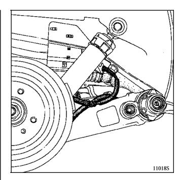
Disconnect the sensor connector located under the vehicle.
