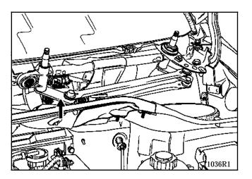
Disconnect and release the motor connector.
