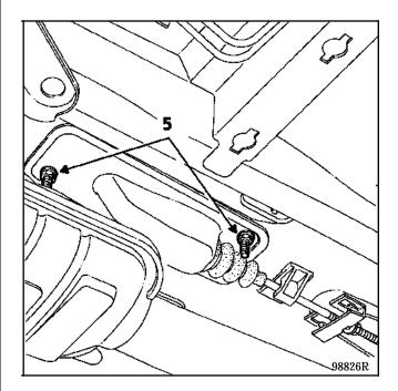
Remove the handbrake lever from under the vehicle.
