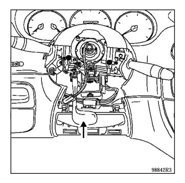
**IMPORTANT:** to remove the dashboard, the steering column height adjustment handle must be released.
