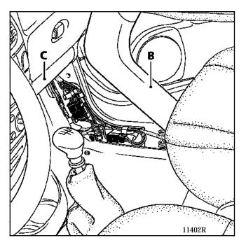
Remove the insulating foam under the fan.
