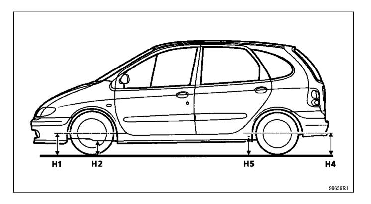
Dimension H5 is measured from the suspension arm axis.
