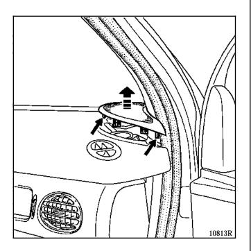
Unclip the speaker grilles and release the centring devices.
