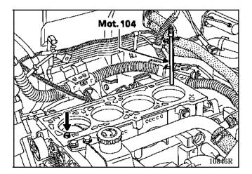
Removal and refitting of the cylinder head gasket is identical to that for the B version for the F3R engine and to N.T. 2526A for the F8Q Turbo engine, except for:
