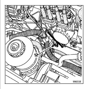
Fit the bracket of tool **Mot. 1159** under the water pump.
