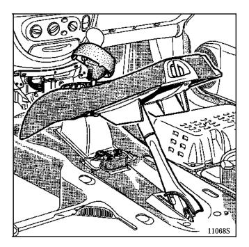
Disconnect the handbrake connector.
