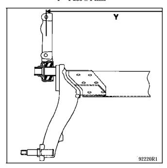
Refit the rear axle assembly to the vehicle and refit the suspension arms (see corresponding section).
