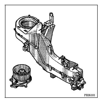
Release the fan assembly, then turn it anticlockwise through  $90^{\circ}$  to remove it.
