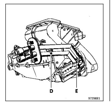
Separate the water downpipe from the heater matrix.
