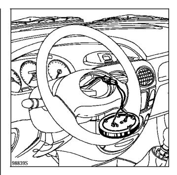
Disconnect the horn assembly and remove it.
