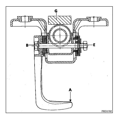
Fit a 15 mm thick shim (G) between the body and the steering column.
