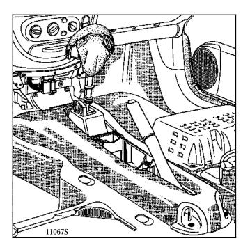
Lift the console to release the handbrake lever.
