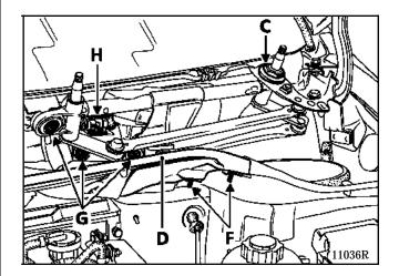
the three bolts (G) mounting the mechanism / motor assembly after disconnecting the motor connector (H).
