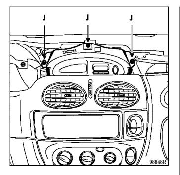
Remove the clock, three bolts (J).
