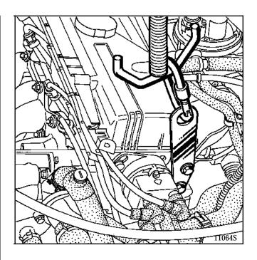
The engine support must be positioned as shown in the diagram, then fit the strap around the windscreen aperture.
