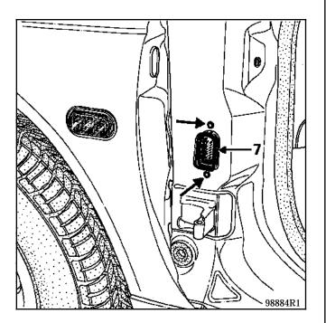
Remove the two bolts for the front door wiring (7), then pass the wiring through into the passenger compartment.
