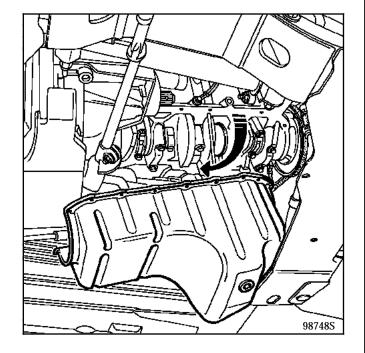
Clean the sump before applying a bead of **RHODORSEAL 5661** of width **3 mm**.
