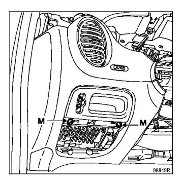
Remove the headlight adjustment unit mounting, two bolts (M).
