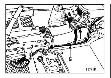
Release the wiring (5) on each side.
