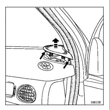
Remove the two mounting bolts for the upper part of the dashboard.
