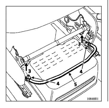
• Partially slacken the two bolts (4) to lift bar (5).
