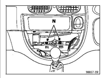
Remove the dashboard mountings on the heating unit, two bolts (N).
