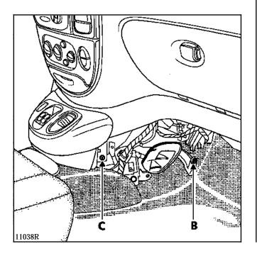
Remove the two mounting bolts (C).
