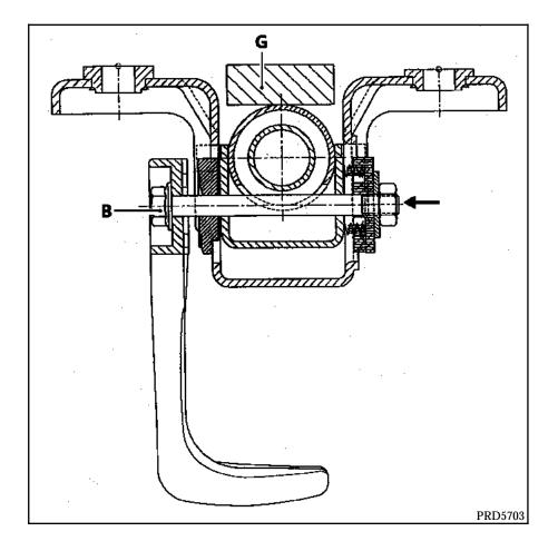
Press on the self locking nut to release bolt (B) to the left.
