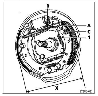
Check the ends of the lower and upper springs are correctly positioned on the shoes.
