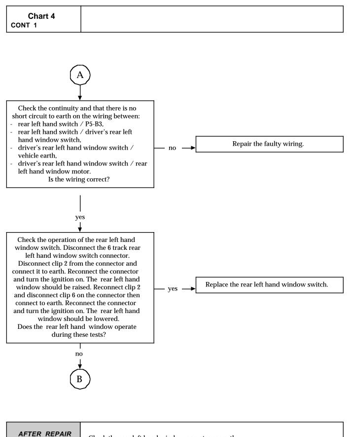
Check the rear left hand window operates correctly.
