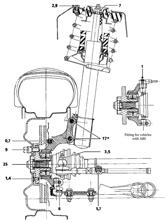
(\*) Fitting direction must be observed (bolt head next to brake caliper)
