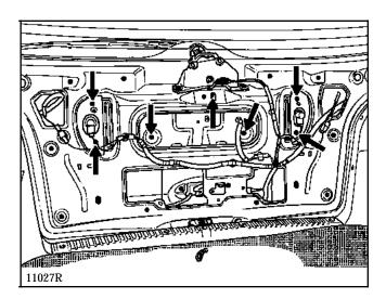
Unclip the strip at (F) and gently separate it from the vehicle to disconnect the connectors for the two number plate lights and release the wiring.
