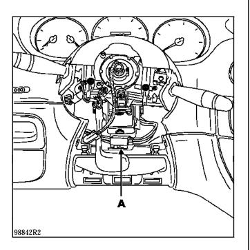
Remove the ignition switch bolt.
