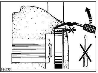
Separate the foam from the steering wheel in the centre, so that tool **Facom D115** may be correctly positioned.
