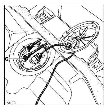
Fit a pipe to empty the pump into a measuring cylinder.
