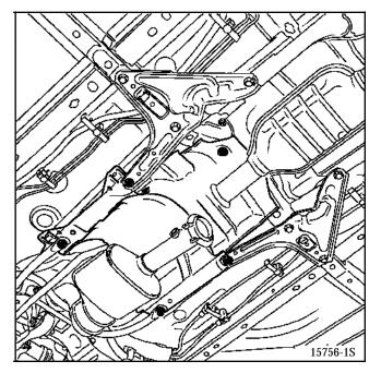
**IMPORTANT:** renew any damaged heat shields to avoid the risk of a fire.
