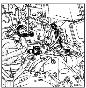
244 Coolant temperature sensor (injection and coolant temperature indication on the instrument panel).
