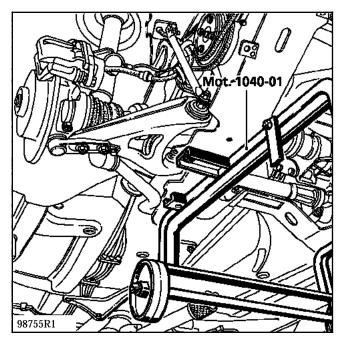
Lower the lift until the tool touches the ground.
