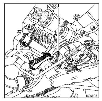
Attach the steering box to the body.
