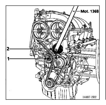
IMPORTANT: all oil must be removed from the head of the crankshaft and the timing sprocket bore and the pressure surfaces of the crankshaft pulley to prevent slip between the timing and the crankshaft which could cause damage to the engine.
