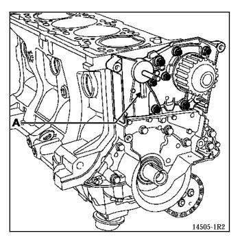
Position the **Renault** logo engraved on the camshaft pulley spokes vertically upright (A), fit the timing belt onto the camshaft pulleys then fit the tool for immobilising the camshaft pulleys **Mot. 1490** (use the timing cover mountings to secure tool **Mot. 1490**).
