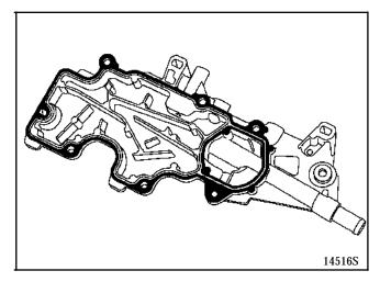
Refit the oil decanter and tighten it to a torque of **1.3 daN.m** in the recommended order.
