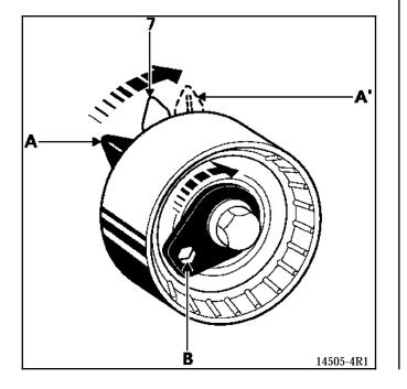
Pre-tighten the tension wheel nut to a torque of **0.7 daN.m**.
