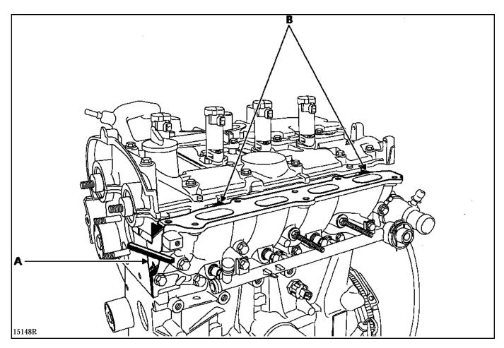
The lower inlet distributor is tightened to a torque of **2.1 daN.m**.
