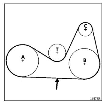
Belt tensioning is carried out using bolt (1) (having slackened the two mounting bolts for the tensioner) then tighten the nut (2).
