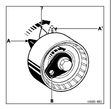
Pre-tighten the tension wheel nut to a torque of **0.7 daN.m**.
