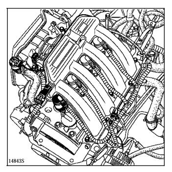
Refitting is the reverse of removal. Observe the tightening torques for the three mounting bolts. Ensure that the O-ring seal is in good condition and that it is correctly fitted.
