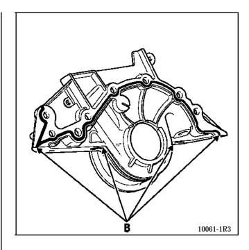
Refit the sump using a new gasket and pretighten it to a torque of **0.8 daN.m**, then tighten in a spiral pattern to a torque of **1.4 daN.m**.
