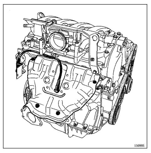
Disconnect and remove the oxygen sensor using Mot. 1495.
