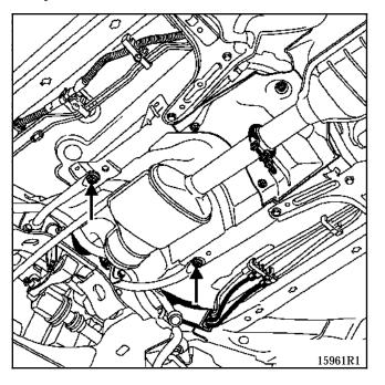
Slacken the four mountings for the sub-frame and fit the dummy sub-frame for removing and refit-ting the engine and transmission assembly.
