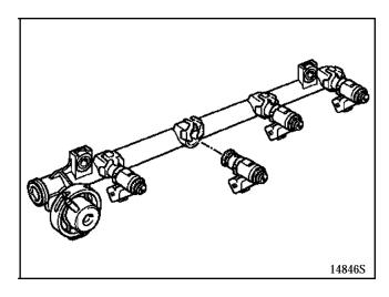
Depending on the vehicle version, the regulator (4) may be located in the engine compartment at the end of the injector gallery (1) or in the fuel tank, on the pump/sender unit assembly. In this case, the end of the gallery, the return union to the fuel tank and the regulator mounting are plugged.
