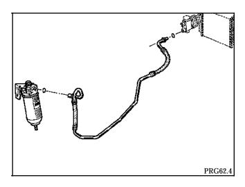
Unclip the pipe from the body then remove it.
