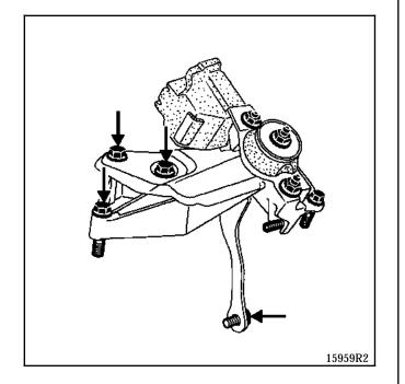
Lower the engine / gearbox assembly.
