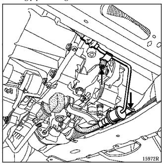
Secure the steering box on the right hand side of the vehicle so that the power assisted steering pipe does not interfere with the removal of the gearbox.
