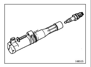
There are four ignition coils and they are mounted directly on the plug by a bolt on the cylinder head cover.
