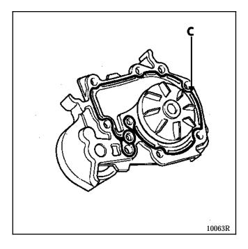
Pretighten bolts M6 and M8 to 0.8 daN.m then tighten M6 bolts to 1.1 daN.m and M8 bolts to 2.2 daN.m in the recommended order.
