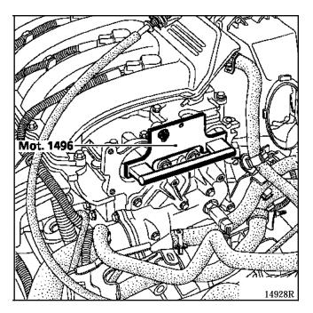
Fit the camshaft pulleys in place by pre-tightening the new nuts (**without locking the nuts, play of 0.5 to 1 mm between nut and pulley**).
