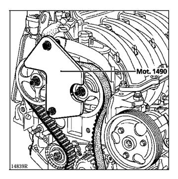
Refit the pulley by tightening the mounting bolt using **Mot. 1368** (to a torque of **4.5 daN.m**, value given for information only).
