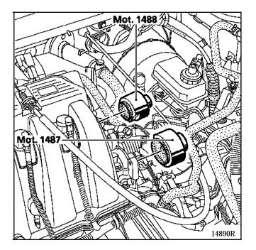
the right hand suspended engine mounting and the engine tie bar, tightening them to the recommended torque (see section 19 "Suspended engine mountings").
