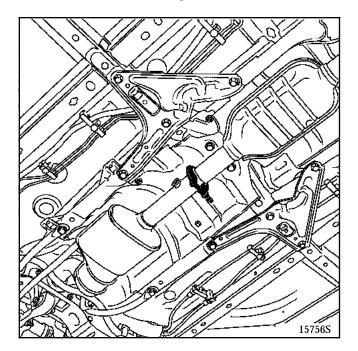
Release the catalytic converter from the silencer pipe.
