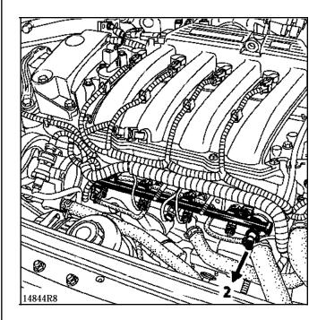
Run the pump using a fault finding tool or by shunting the fuel pump relay (see corresponding wiring diagram).
