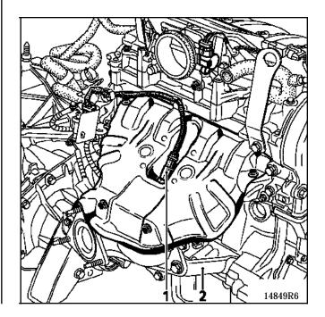
Move the catalytic converter back, without removing it.
