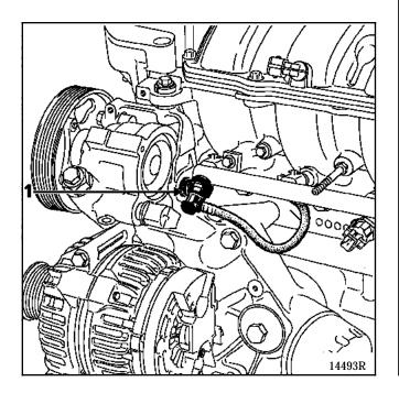
Remove the pump completely (three bolts).
