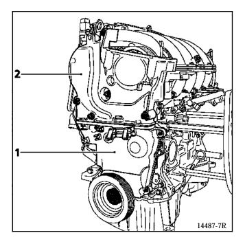
Slacken the timing belt by slackening the tension wheel nut (1).
