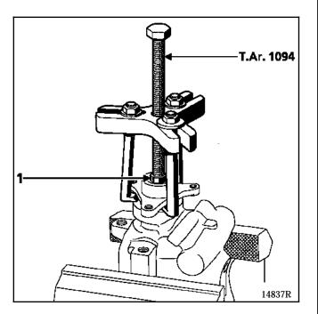
**NOTE:** insert a bolt (1) between the pump shaft and the pushrod of tool **T.Ar. 1094**.
