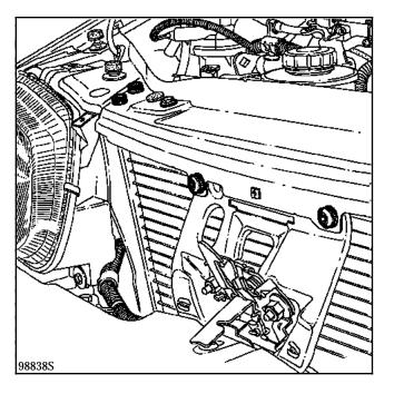
Remove the nut mounting the connecting pipes on the condenser.
