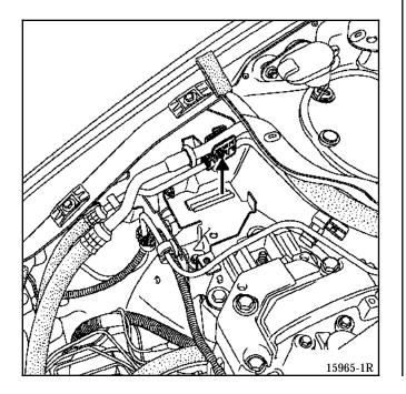
Remove the assembly of low pressure pipes between the expansion valve and the quick release union and the high pressure pipe between the expansion valve and the dehydration canister.
