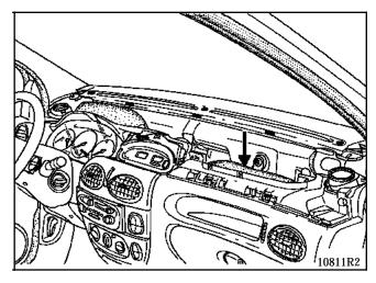
Disconnect the micromotor connector then remove its two mounting bolts.
