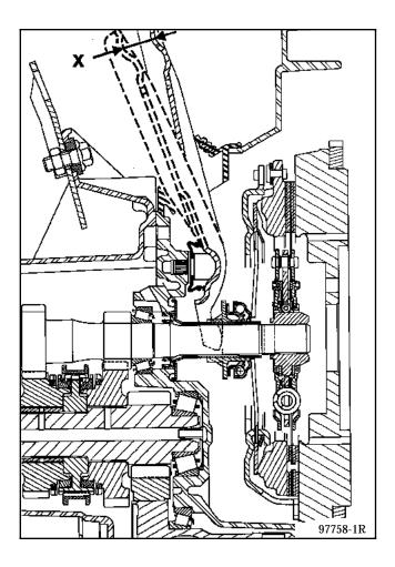
**NOTE:** when an operation does not require removal of the gearbox or after it is fitted, **DO NOT LIFT** the fork as it may become detached from the notch (A) of the thrust bearing.
