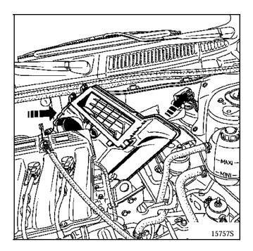
**NOTE** : take care with the vacuum outlet from the inlet manifold to the braking amplifier. If this outlet is broken, the manifold must be replaced.
