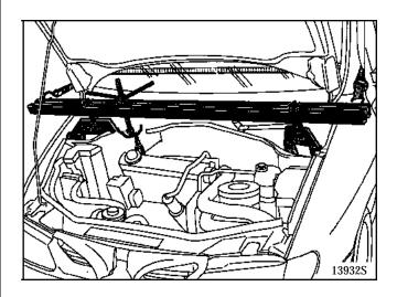
Remove the suspended engine mounting cover.
