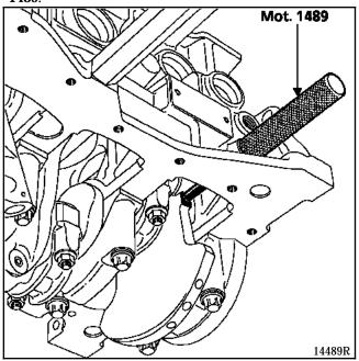
Tighten the crankshaft accessories pulley bolt to a torque of **2 daN.m**, then to an angle of  $135^{\circ} \pm 15^{\circ}$  (crankshaft touching the TDC pin).
