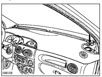
Remove the front right hand vent duct.
