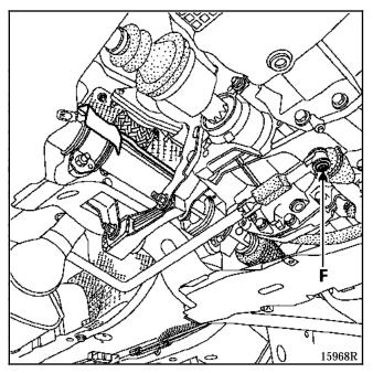
Remove the gear control linkage.
