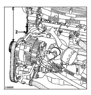
NOTE : the accessories belt has five teeth whilst the alternator, PAS pump and crankshaft pulleys have six; it is therefore essential to ensure that the tooth at the end of the pulleys (E) remains "free" when refitting the belt.
