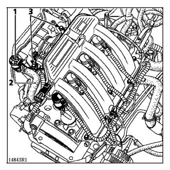
Move the air unit to the right to remove it. The air unit may go between the windscreen aperture, the engine and the braking amplifier.
