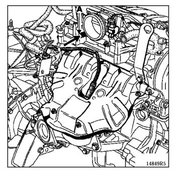
Oil vapour recuperation plate located on the cylinder head cover.
