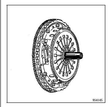
Gradually tighten in a star pattern then torque tighten the mechanism mounting bolts.
