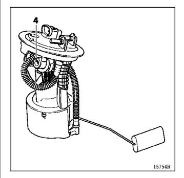
**NOTE** : for vehicles operating without a pipe returning fuel from the engine to the tank, the pressure regulator (4) is located on the pump and sender unit assembly. It cannot be removed.
