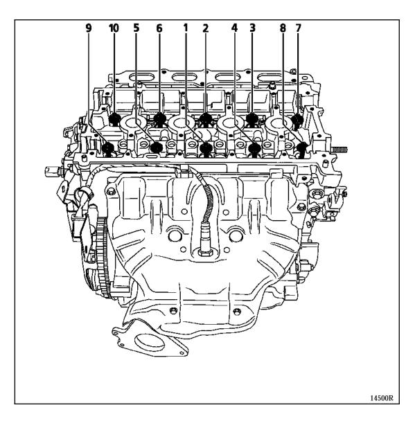
Check that all bolts are tightened to a torque of **2** daN.m then angle tighten (bolt by bolt) to  $240^{\circ} \pm 6^{\circ}$ .
