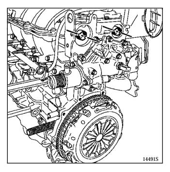
Insert the Top Dead Centre pin **Mot. 1489** then rotate the engine clockwise (timing side) to slowly and without jerky movements, bring the crankshaft into contact with the pin.
