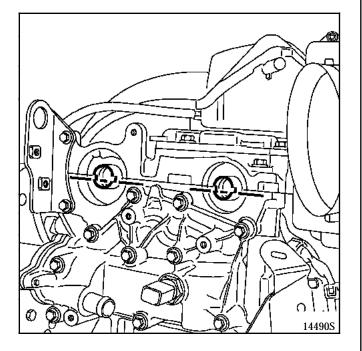
Fit tool Mot. 1496 to the end of the camshafts.
